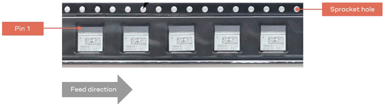
Figure 7: Orientation of ANNA-B112 modules on tape
